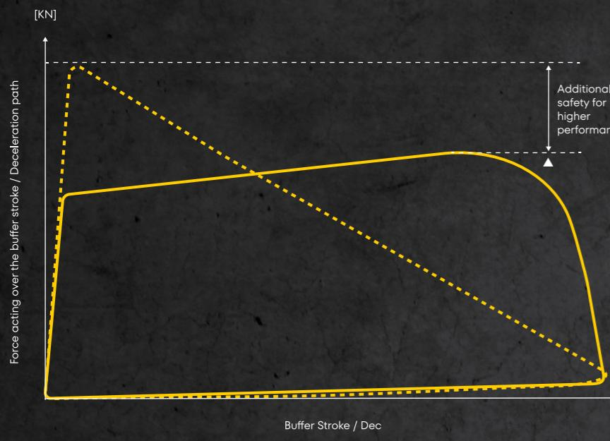
Many COMPETITORS provide hydraulic buffers with limited impact mass capacity, which may result in reduced performance and safety in more demanding applications
